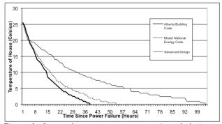
Figure 1: Lowest house temperature experienced during a power failure by failure duration and house design for the City of Edmonton.
